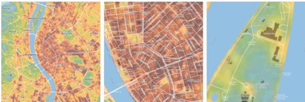
Figure 60: Hyper-resolution (10 m) temperature map of Budapest on September 6, 2023, at 04:00h . The temperature spread at that time was 14 °C (blueish) to 19 °C (dark brown).
